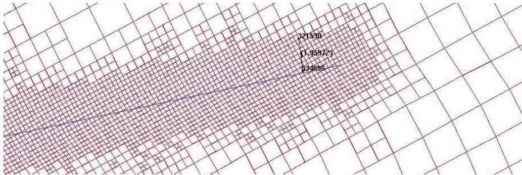
Figure 15-24. Mesh refinement with TCTOL=2.0
