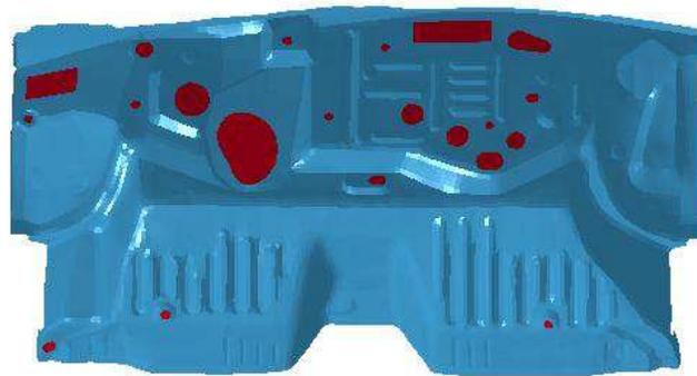
Figure 12-8. Trimmed-out holes dilled with LS-PrePost
