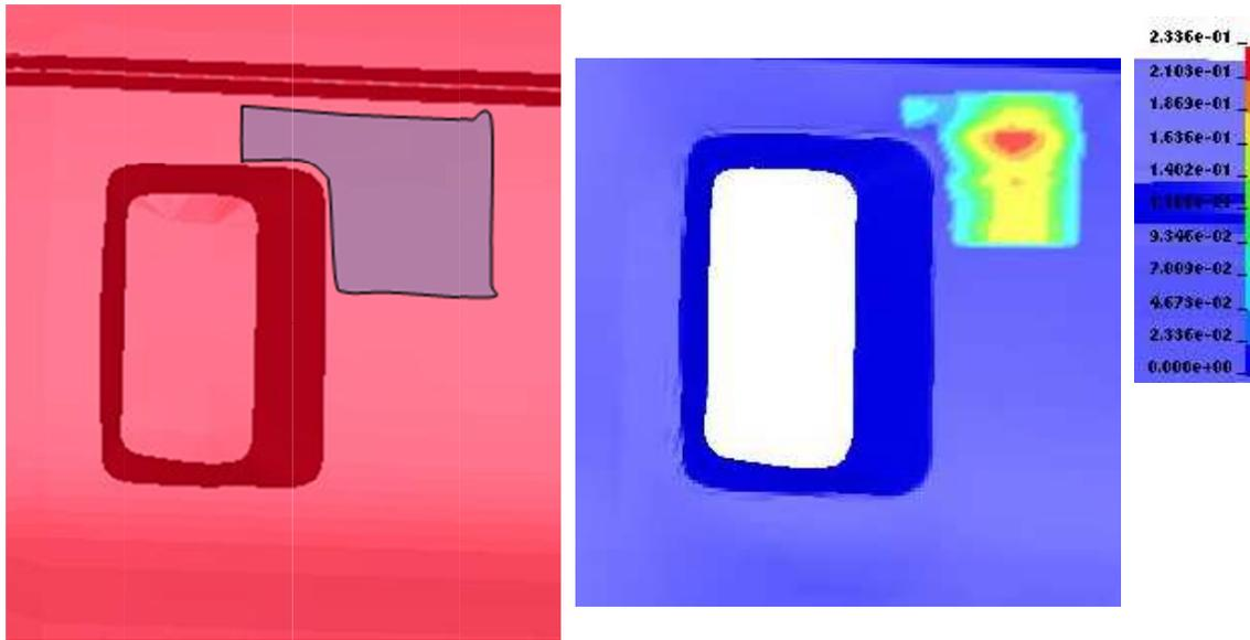
Figure 12-26. The element sets selected for stoning/Stoning results.
