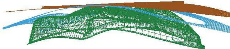
Figure 12-18. Gravity loaded blank without using this keyword –Blank sags in the die cavity (concave shape)
