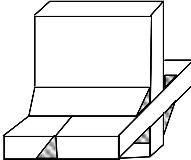
Figure 10-9. A combined weld is a mixture of fillet and butt welds.
