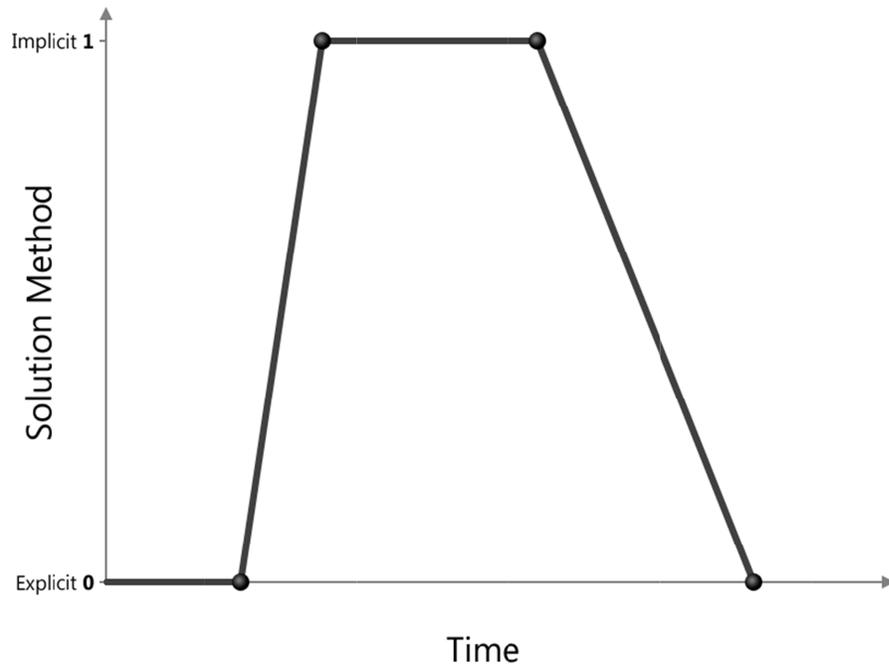
Figure 12-49. Solution method, implicit or explicit, controlled by a load curve.
