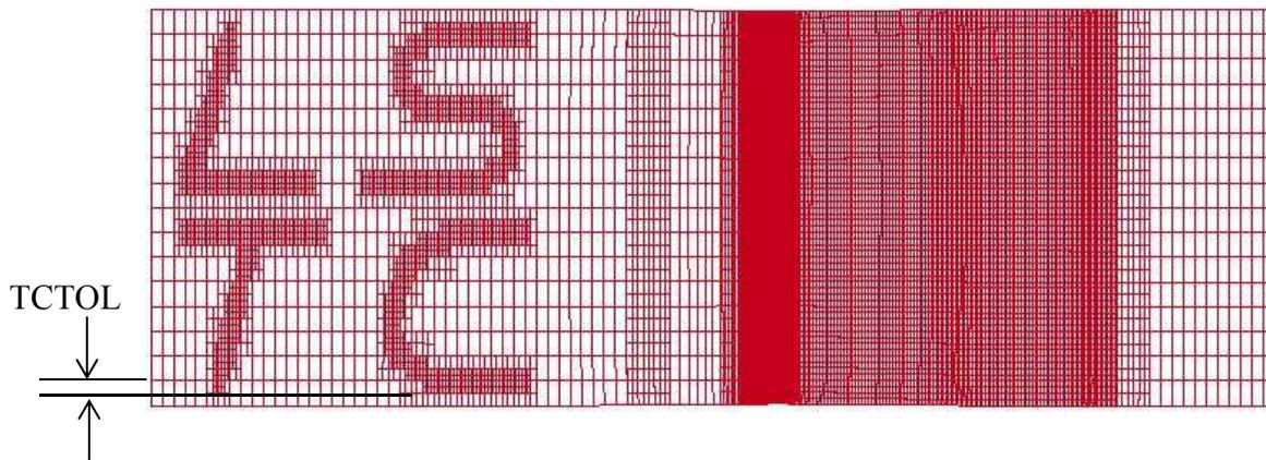
Figure 15-19. Define the variable TCTOL to limit the mesh adaptivity area.
