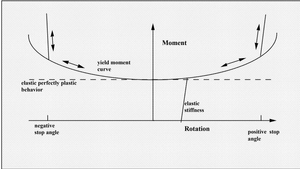
Figure 10-24. Frictional behavior is modeled by a plasticity model. Elastic behavior is obtained once the stop angles are reached. The same elastic stiffness is used to simulate sticking situations.
