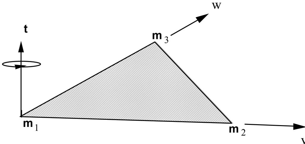
Figure 27-4. Follower force and moment acting on a plane defined by nodes  $m_1$ ,  $m_2$ , and  $m_3$ . In this case, the load is applied to node  $m_1$ ; i.e.,  $m=m_1$ . A positive force acts in the positive  $t$ -direction, and a positive moment puts a counterclockwise torque about the normal vector. The positive  $t$ -direction is found by the cross product  $t = v \times w$  where  $v$  and  $w$  are vectors as shown.
