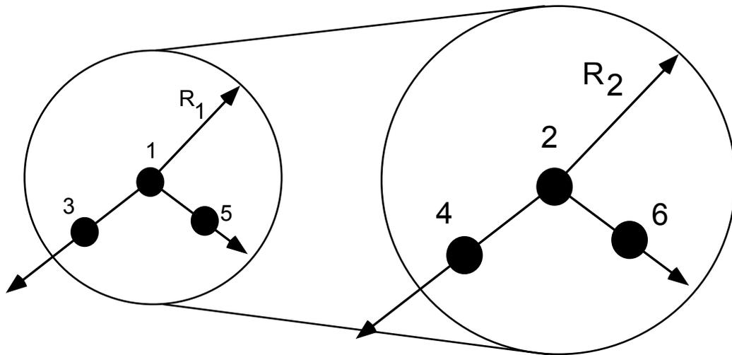
Figure 10-20. Pulley joint. Nodal pairs (1,3) and (2,4) define axes that are orthogonal to the pulleys. Nodal pairs (1,5) and (2,6) define vectors in the plane of the pulleys. The ratio  $\frac{R_2}{R_1}$  is specified.
