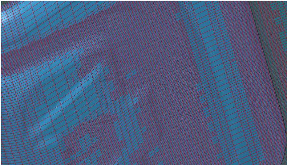
Figure 12-41. Binder closing with adaptive refinement on a decklid inner (NNU-MISHEET'05)
