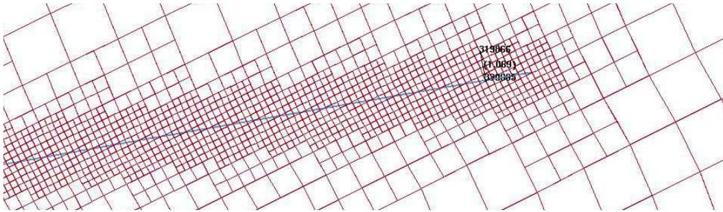
Figure 15-23. Mesh refinement with TCTOL=1.0
