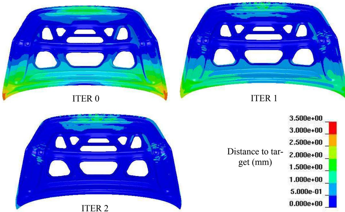
Figure 25-25. Iterative compensation for a localized region
