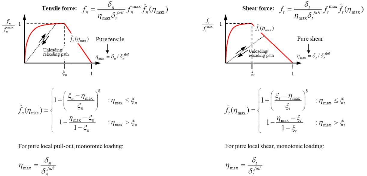
Figure 10-35. Force-deformation relationship: non-linear damage model.
