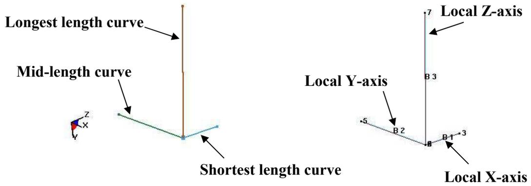
Figure 15-3. Input curves. Generated local coordinate system beams when viewed in LS-PrePost (right)
