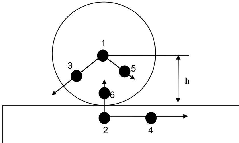
Figure 10-18. Rack and pinion joint. Nodal pair (1,3) defines the axis of rotation of the first body (the pinion). Nodal pair (1,5) is a vector in the plane of the pinion and is orthogonal to nodal pair (1,3). Nodal pair (2,4) defines the direction of travel for the second body (the rack). Nodal pair (2,6) is parallel to the axis of the pinion and is thus parallel to nodal pair (1,3). The value  $h$  is specified. The velocity of the rack is  $\omega_{pinion} \times h$ .
