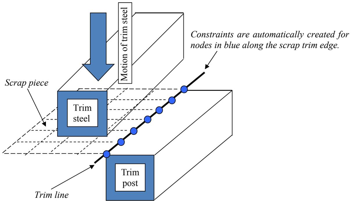
Figure 12-21. Simulation initialization (Courtesy of Ford Motor Company)
