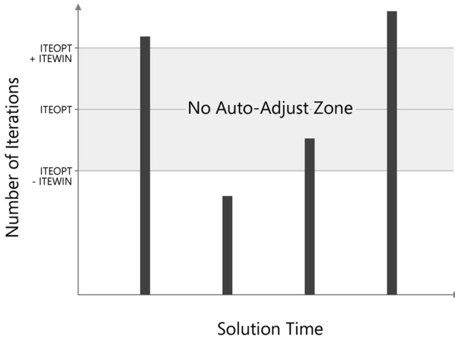
Figure 12-32. Iteration Window as defined by ITEOPT and ITEWIN.
