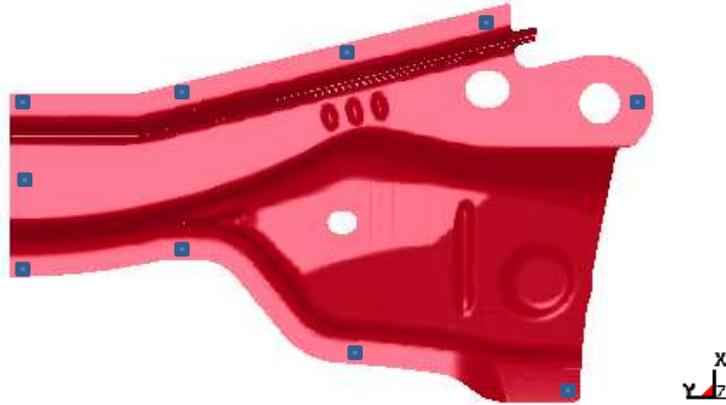
Figure 10-2. Constrained locations of a springback panel (NUMISHEET 2005 cross member).
