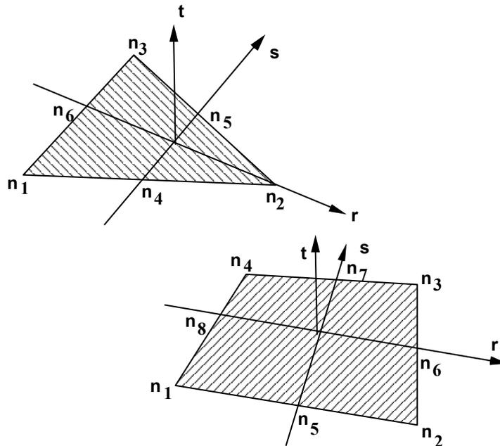
Figure 27-5. Nodal numbering for pressure segments in three-dimensional geometries. Positive pressure acts in the negative t-direction.
