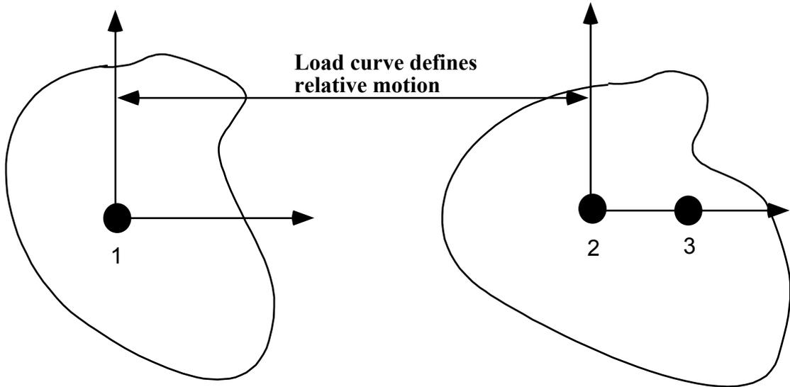
Figure 10-15. Translational motor joint. This joint can be used in combination with the translational or the cylindrical joint.
