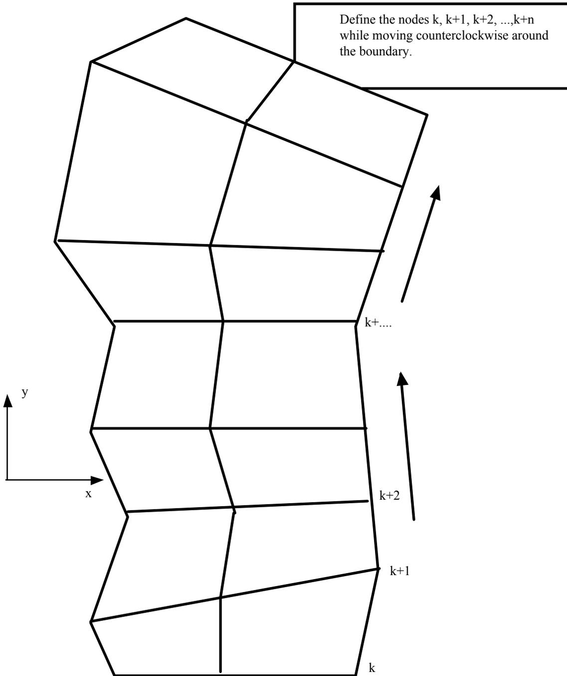
Figure 5-3. When defining a transmitting boundary in 2D define the node numbers in the node set in consecutive order while moving counterclockwise around the boundary.
