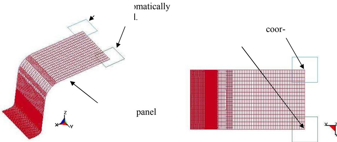
Figure 12-3. Two examples are shown in the following figure, where a trimmed blank is gravity loaded in -Z direction and in +Z direction and the corresponding springback shapes are calculated.
