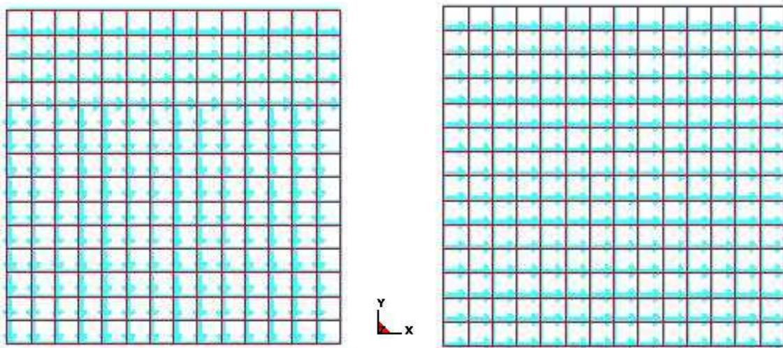
Figure 15-33. Element direction (N1-N2) of incoming sheet blank (left) and after re-orientation.
