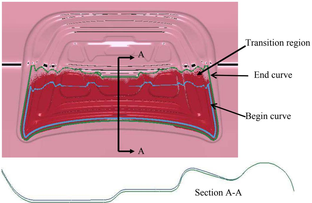
Figure 25-24. Two curves defining a localized compensation zone of the upper half of the deck lid
