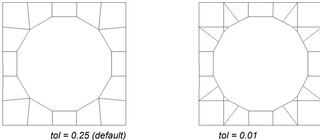
Figure 15-17. Trimming Tolerance. The tolerance limits the size of the small elements generated during trimming. The default tolerance (left) produces large elements. Using a tolerance of 0.01 (right) allows smaller elements, and more detail in the trim line.
