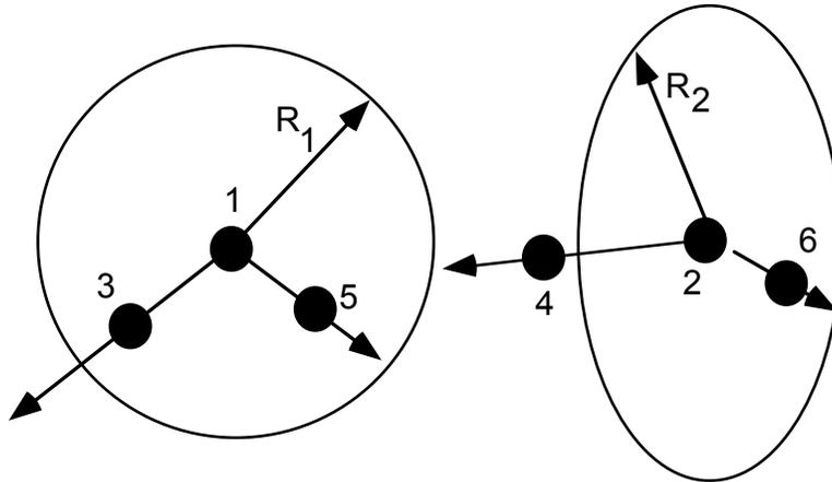
Figure 10-17. Gear joint. Nodal pairs (1,3) and (2,4) define axes that are orthogonal to the gears. Nodal pairs (1,5) and (2,6) define vectors in the plane of the gears. The ratio  $\frac{R_2}{R_1}$  is specified.
