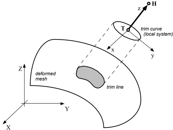
Figure 15-16. Trimming Orientation Vector. The tail (T) and head (H) points define a local coordinate system (x,y,z). The global coordinate system is named (X,Y,Z). The local x-direction is constructed in the Xz plane. If X and z nearly coincide ( $|X \cdot z| > 0.95$ ), then the local x-direction is instead constructed in the Yz plane. Trim curve data is input in the x-y plane, and projected in the z-direction onto the deformed mesh to obtain the trim line.
