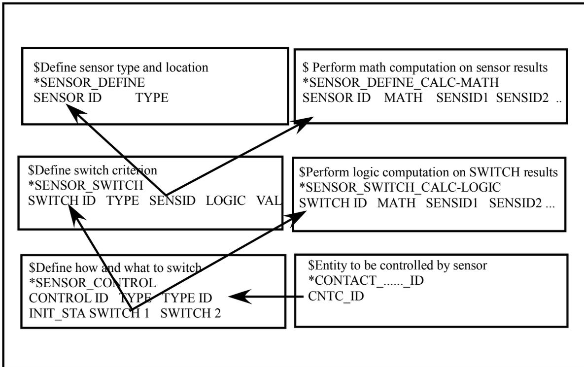
Figure 35-1. Relationship between sensor keyword definitions.
