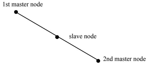
Figure 4-2 This simple constraint, which ensures that a slave node remains on a straight line between two master nodes, is sometimes necessary during ALE smoothing.
