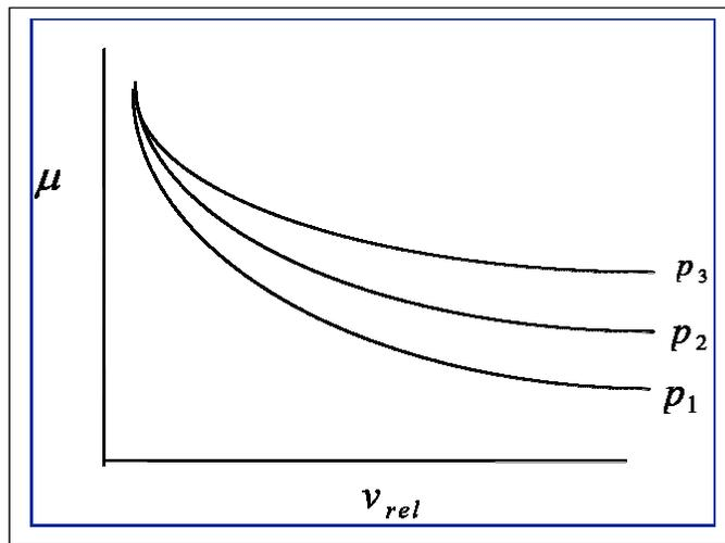
Figure 11-1. Friction coefficient,  $\mu$ , can be a function of relative velocity and pressure. Specify a flag for the static coefficient of friction, FS, and a table ID for the dynamic coefficient.
