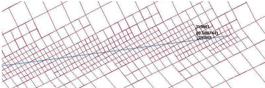
Figure 15-22. Mesh refinement with TCTOL=0.5.
