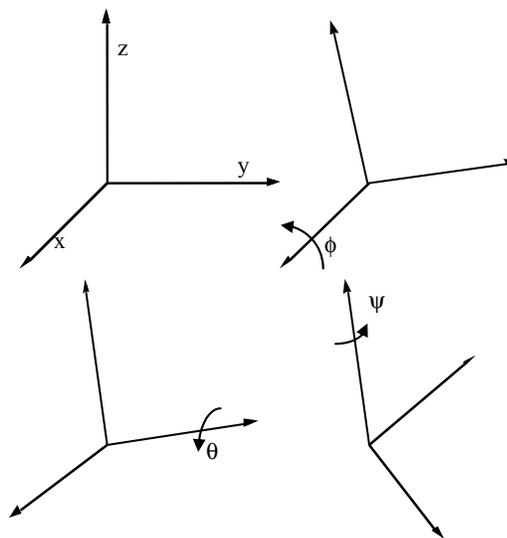
Figure 10-23. Definition of angles for the generalized joint stiffness.
