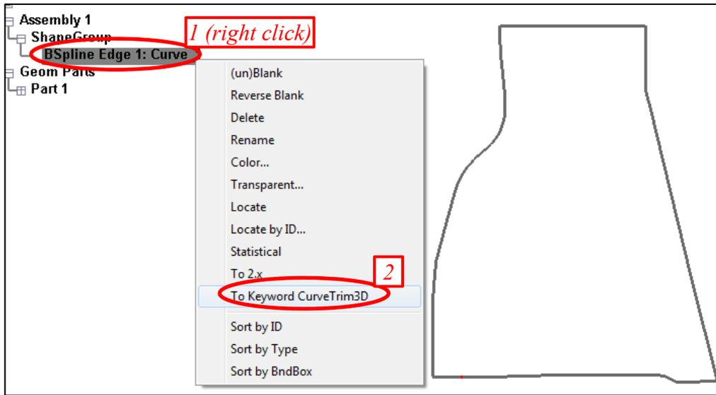
Figure 25-2. To convert back and forth between IGES curves and XYZ format to be used for \*DEFINE\_TARGET\_BOUNDARY, menu option *Curve/Covert (Curve)/To XYZ file*, or *From XYZ file* can be used.
