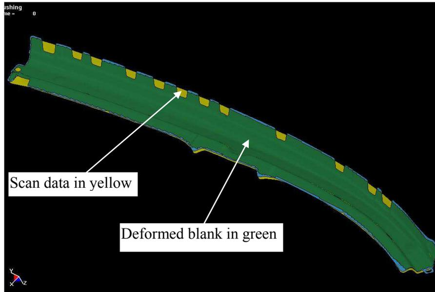
Figure 25-22. A trimmed panel “pushed” onto the scan data (rigid body)
