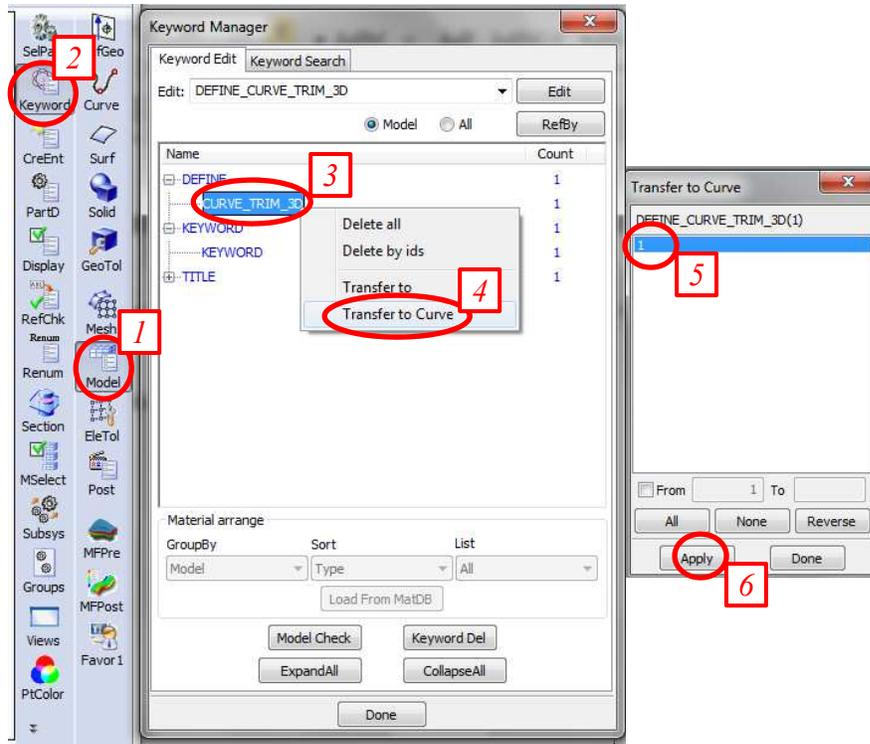
Figure 25-1. Converting *trimcurves.ibo* to IGES format in LSPP4.0
