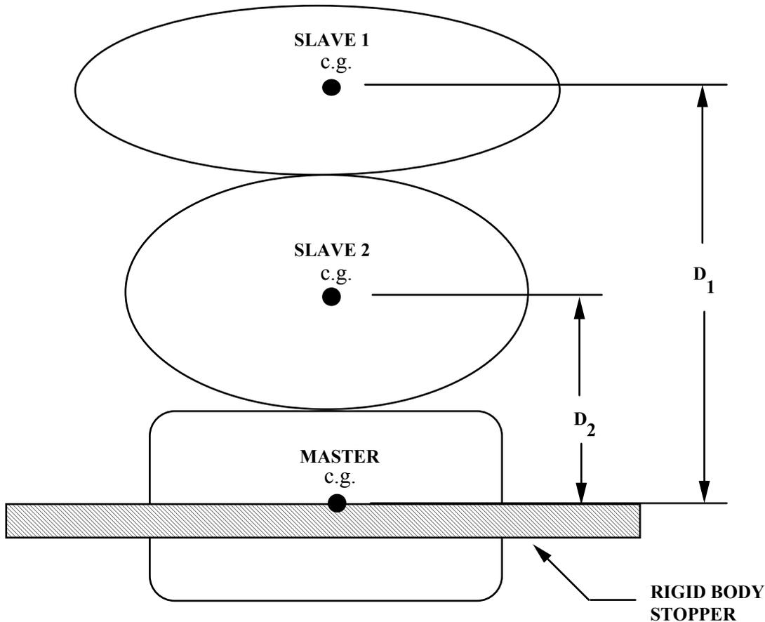
Figure 10-29. When the master rigid body reaches the rigid body stopper, the velocity component into the stopper is set to zero. Slave rigid bodies 1 and 2 also stop if the distance between their mass centers and the master rigid body is less than or equal to the input values  $D_1$  and  $D_2$ , respectively. (c.g. + center of gravity).
