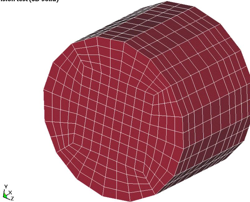
Figure 44-1. Solid mesh for user element test.
