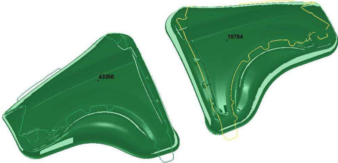
Figure 15-11. Using the two nodes from the stationary tools at its home position to define NSEED1 and NSEED2 for trimming of a double-attached part (NUMISH-EET2002 Fender Outer)
