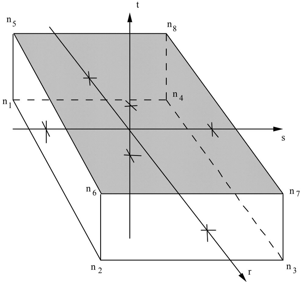
Figure 18-21. 8-node Thick Shell Element.
