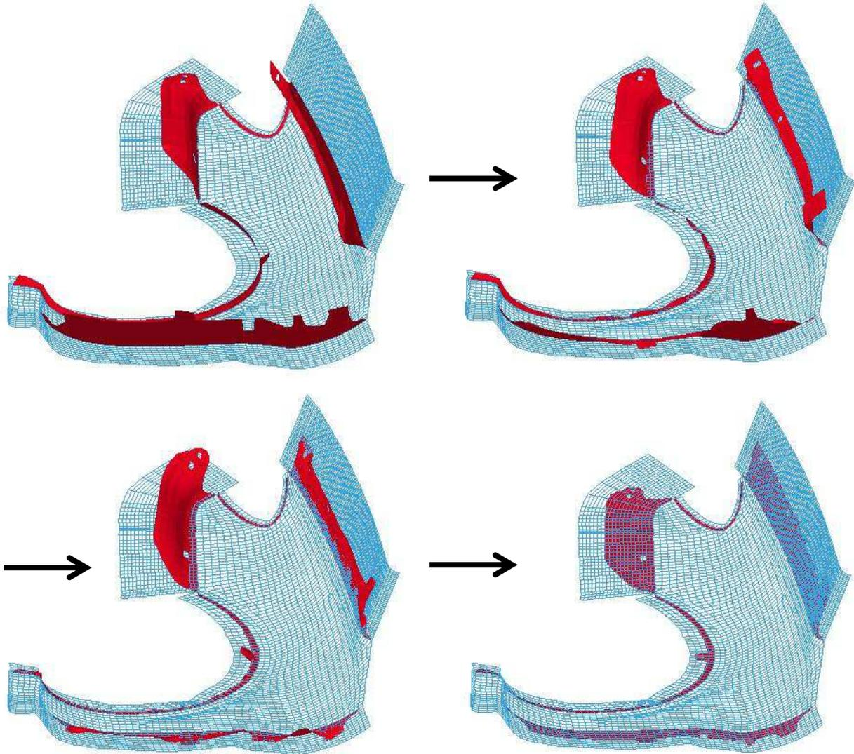
Flange unfolding progression of a fender outer
