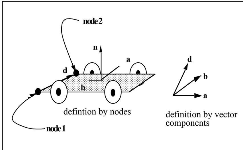
Figure 33-2. Definition of orthotropic friction vectors. The two methods of defining the vector,  $\mathbf{d}$ , are shown. If vector  $\mathbf{d}$  is defined by nodes 1 and 2, the local coordinate system may rotate with the body which contains the nodes; otherwise,  $\mathbf{d}$  is fixed in space, thus on the rigid wall, and the local system is stationary.
