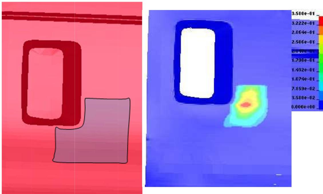
Figure 12-27. The element sets selected for stoning/Stoning results.
