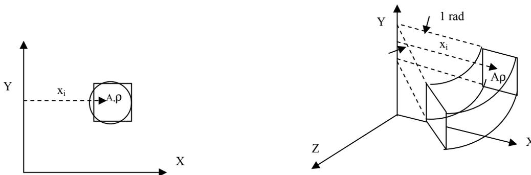
Figure 18-20. An axisymmetric SPH and corresponding shell Mass printout in d3hsp, mass/radian
