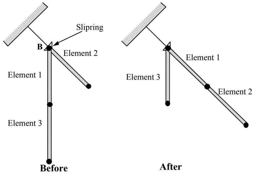
Figure 18-10. Elements passing through slipping.
