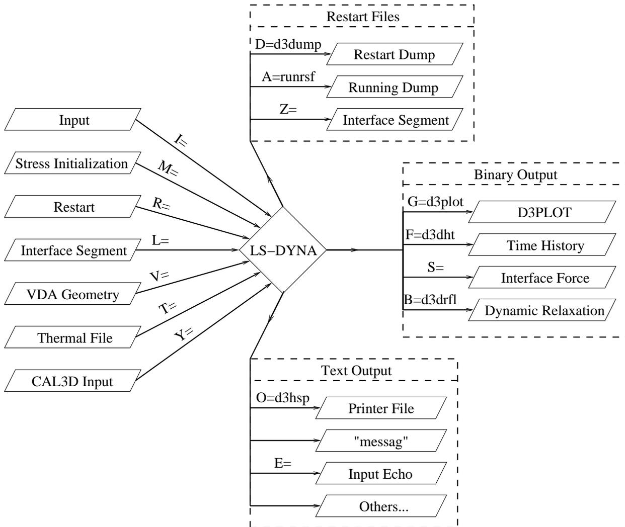
Figure 2-2. Files Input and Output.
