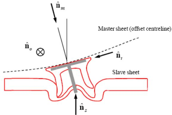
Figure 10-31. Plane of maximum opening.
