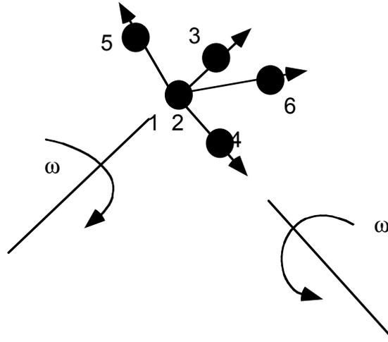
Figure 10-19. Constant velocity joint. Nodal pairs (1,3) and (2,4) define an axes for the constant angular velocity, and nodal pairs (1,5) are orthogonal vectors. Here nodal points 1 and 2 must be coincident.
