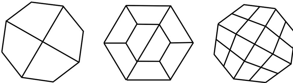
Figure 15-36. Sample four, eight, and sixteen element spot weld clusters comprised of solid hexahedron elements.
