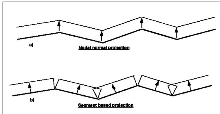
Figure 11-10. Nodal normal and segment based projection is used in the contact options
