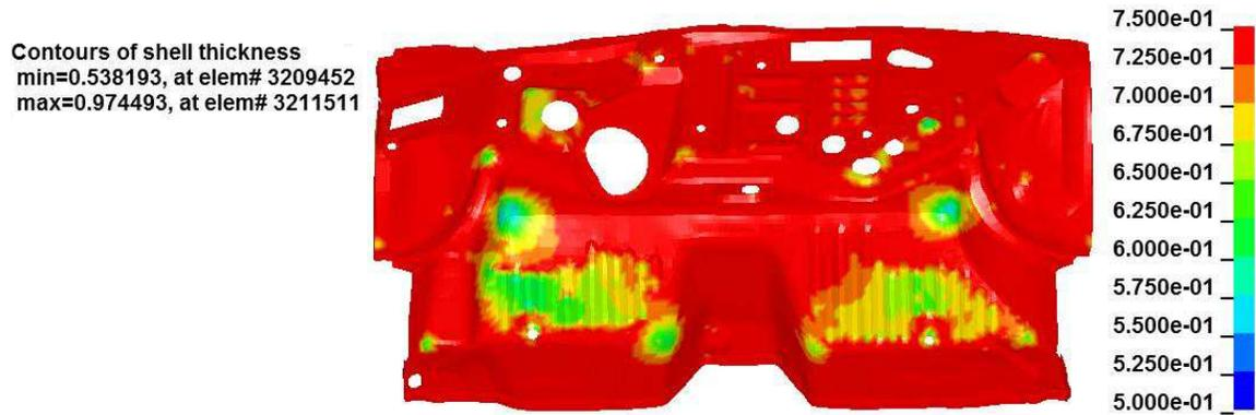
*Blank thickness without holes ( $t_0=0.75\text{mm}$ )*
