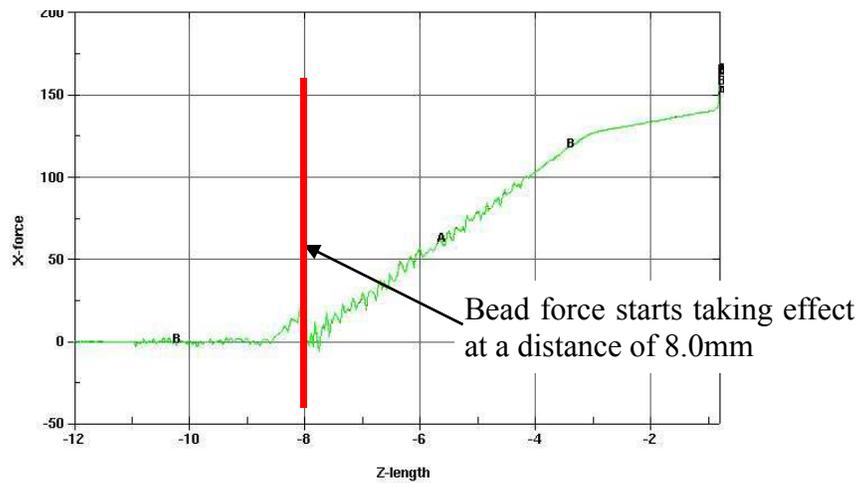
Figure 11-5. Pulling force (NODFOR) vs. closure distance.
