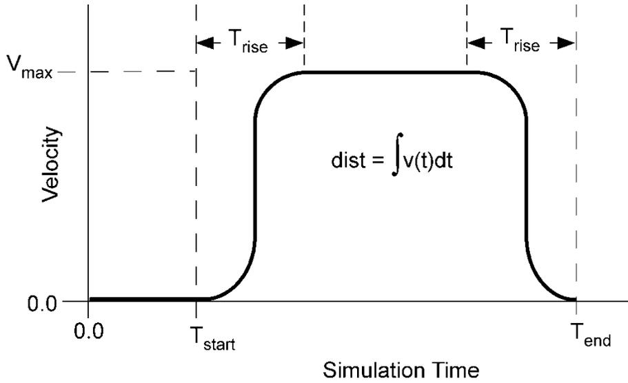
Figure 15-10. Smooth curve created automatically using \*DEFINE\_CURVE\_SMOOTH. This shape is commonly used to control velocity of tools in metal forming applications as shown in the above graph, but can be used for other applications in place of any standard load curve.
