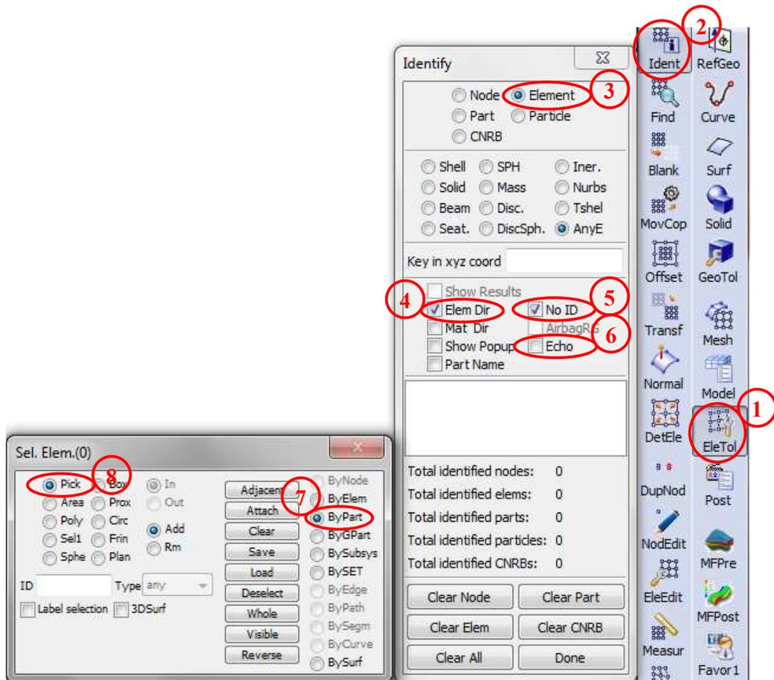
Figure 15-34. Checking element directions (N1-N2) by part using LS-PrePost4.0
