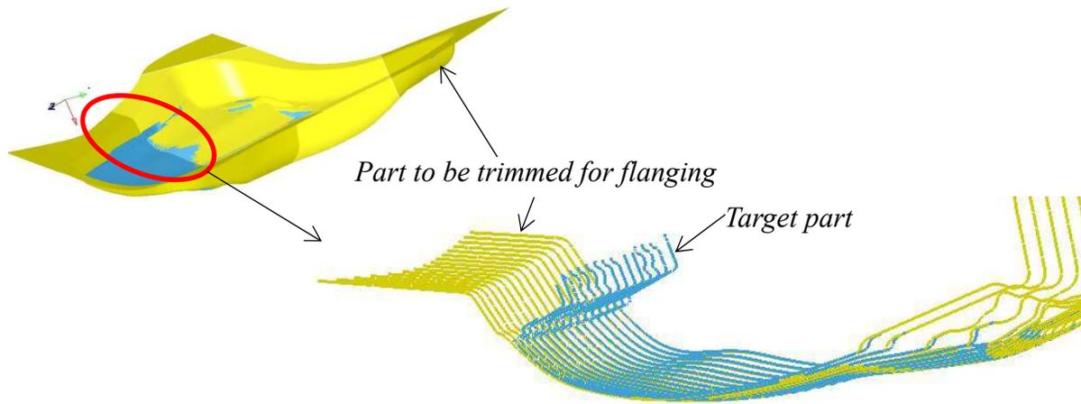
Figure 25-13. Multiple section view showing target part and addendum surfaces
