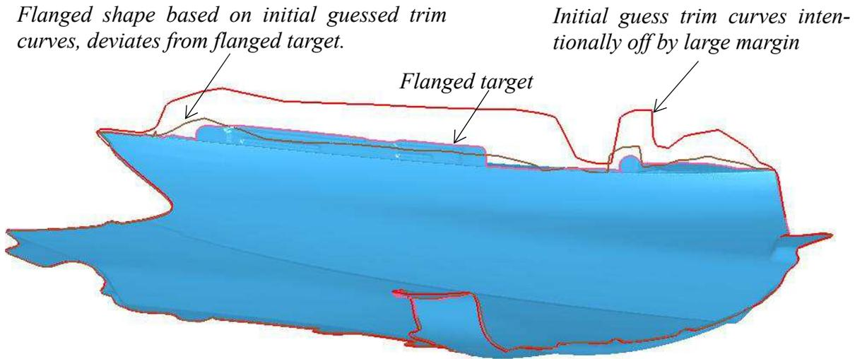
Figure 25-15. Initial trim curves intentionally made to be off by large margin.
