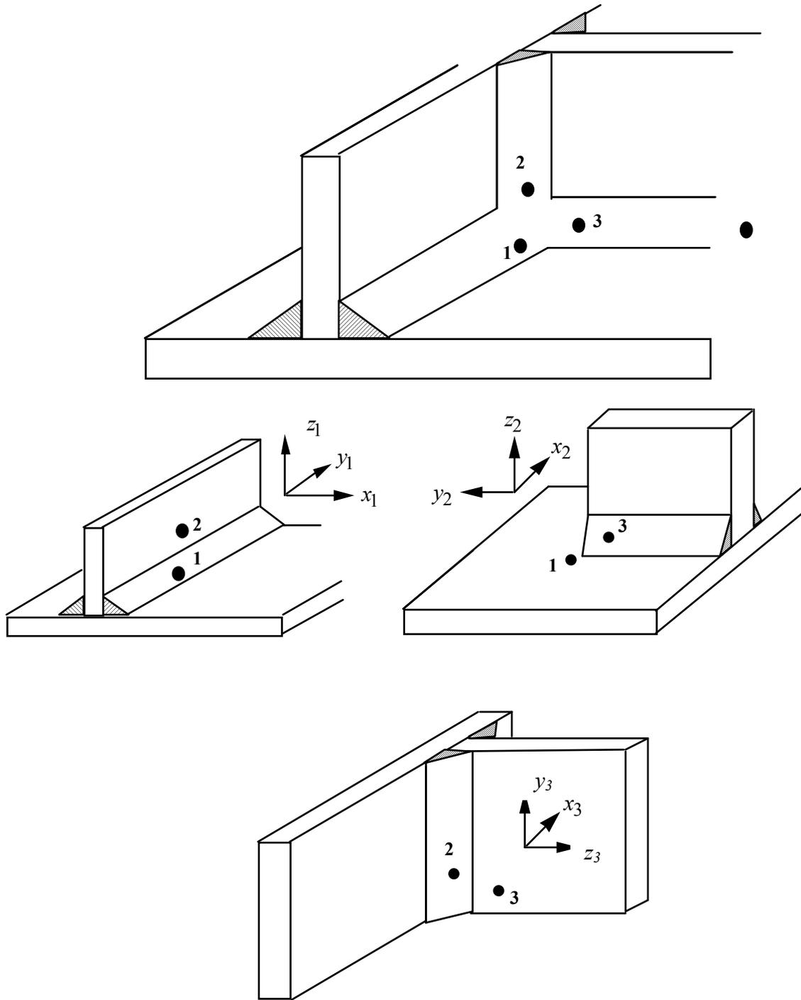
Figure 10-8. A simple cross fillet weld illustrates the required input. Here NPR=3 with nodal pairs (A=2, B=1), (A=3, B=1), and (A=3, B=2). The local coordinate axes are shown. These axes are fixed in the rigid body and are referenced to the local rigid body coordinate system which tracks the rigid body rotation.
