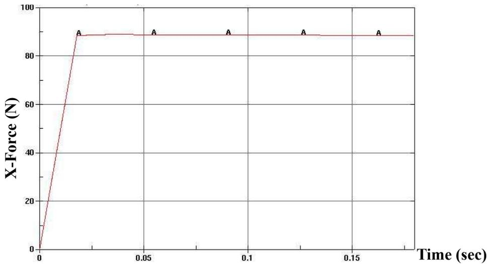
Figure 15-35. Pulling force (frictional force) from RCFORC file.
