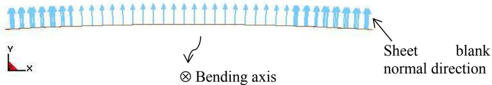
Figure 12-15. Negative “R” means center of bending is on the opposite side of the positive blank normal
