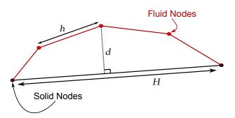
Figure 5-1. Geometry of FSI contact.
