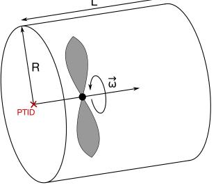
Figure 5-2. Non Inertial Reference Frame Example
