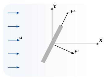
**Figure 5-3.** Anisotropic porous media vectors definition (PMMID = 4). The vectors **X** and **Y** are the global axes; **x**' and **y**' define system for the primed coordinate (x', y', z').
