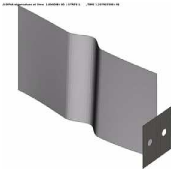
Figure 12. The lowest buckling mode shape for the panel.
