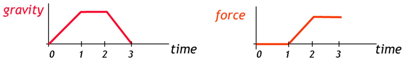
Figure 2. Definition of multiple load cases for linear static analyses. Each time ( t=1, 2, \dots ) corresponds to a new load case. Note that \Delta t = 1 .
