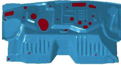
Trimmed-out Holes Filled with LS-PrePost
