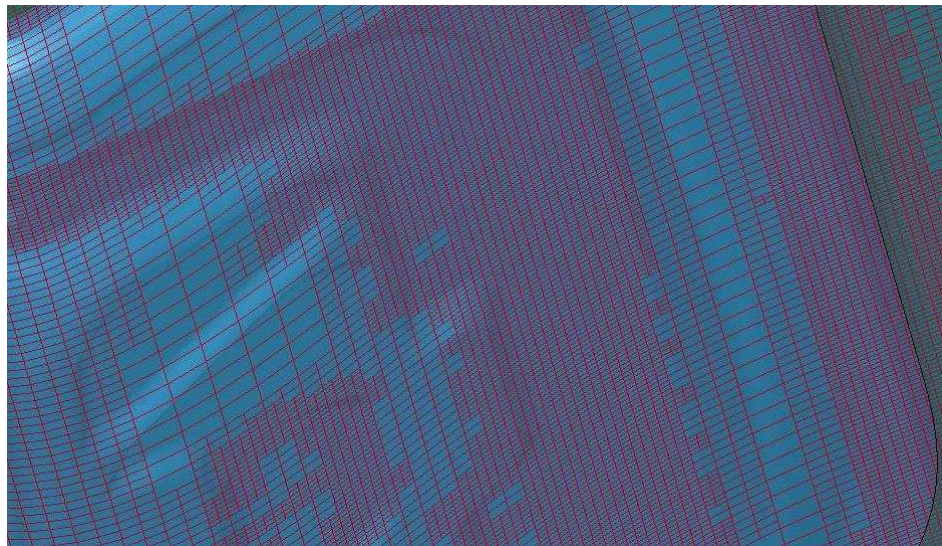
Binder closing with adaptive refinement on a decklid inner (NNUMISHEET'05)
